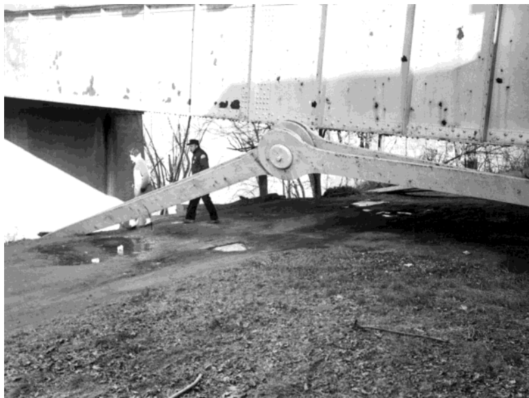
A failed eyebar beneath the collapsed Silver Bridge.
